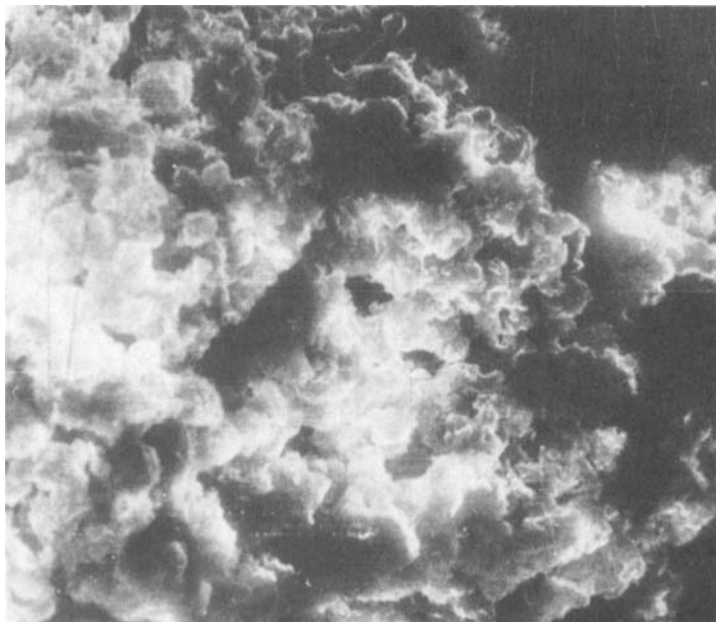
FIG. 4. Scanning electron micrograph of a polyacrylamide sample obtained by polymerization using MYRJ 45 as emulsifier. Sample prepared by graphite deposition. 250 \times .
